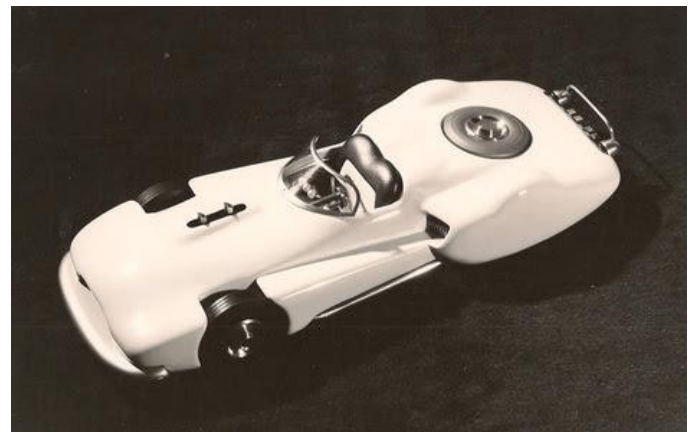
The exposed top of the front wheels in the design was most probably due to comments from Tremulis' long-time friend, Ab Jenkins, who thought you had to see how the tread was wearing on the tires and how the suspension was handling the roadway - especially important for racing.
