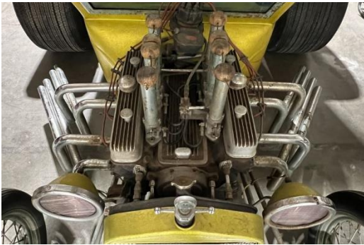
Wooden plugs keep mice out of the stacks on the fuel-injected Buick V8
