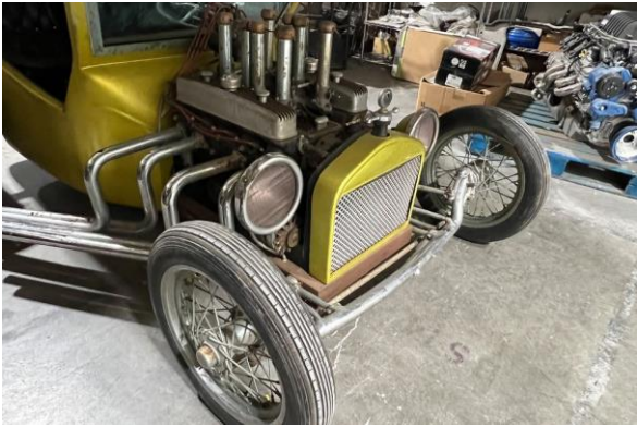
one of the few actual Model T parts on the car is the radiator shell, probably off a '23-'27 Ford.
