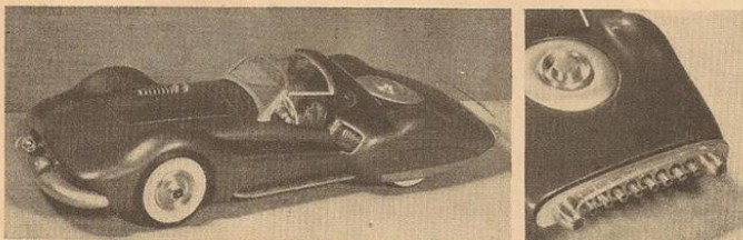
Fig. 10. Model of Tremulis' sports car design has 2 air intake tubes atop the hood, intake at front of rear fenders to increase brake cooling, spare tire mounted on top of rear deck and a row of exhaust pipes at the tail (shown at right). This car would be in the 135-150 mph class.
