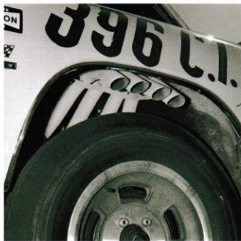
> Not normally seen in photos of the Chevelle are the individual exhaust pipes dumping into the wheelhouse above the front tires on what appear to be real magnesium wheels, which mix well with fire. Power was from a stock 396ci and four-speed. Drag Axle-equipped cars could drive around under normal power from a mundane V8.
