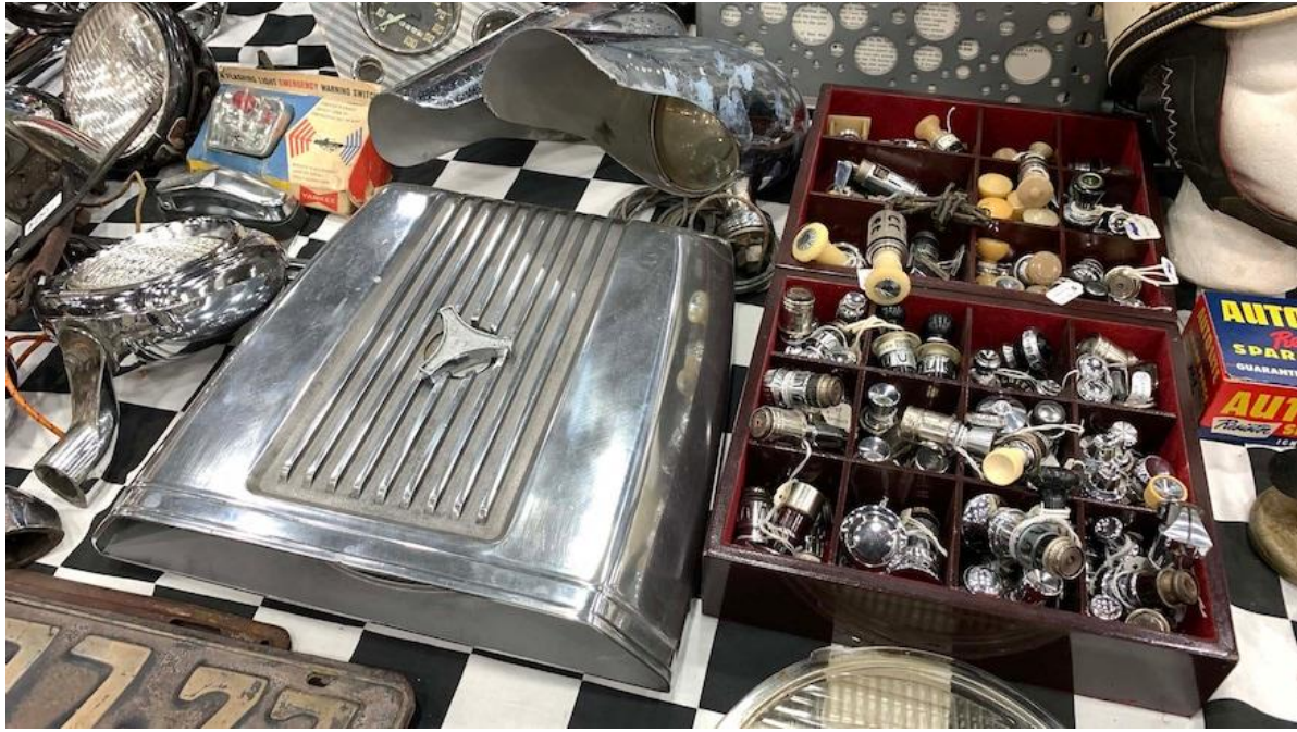
On the left is a Cal Custom air cleaner scoop from the '60s. To the right, an assortment of lighters, mostly from the '50s and '60s. Lighters were a component in virtually every car from that era but frequently disappear from cars, so replacements are popular with restorers. Several of these feature Bakelite knobs.
