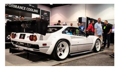
Rotiform worked with Burroughs to create his ideal wheel set up that fit perfectly over AP brakes, H&R Springs built coilovers to his provided specs, and everything around those pieces is entirely custom. The engine compartment, a point of disdain for Burroughs at Ferrari's lack of detail and finish work from the factory, was lambasted then sandblasted and painted at the StanceWorks shop, and later its outside given a bright white makeover by All City Wraps.
